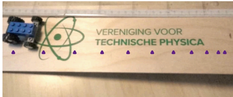
Figure 2.5: Calculating velocity requires both position and time, both easily measured e.g. using a stopmotion where one determines the position of the car per frame given a constant time interval.
