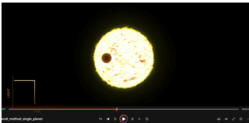
Figure 2.175: Changing intensity of star light due to a period passage of a planet orbiting the star ( animation from NASA ).
