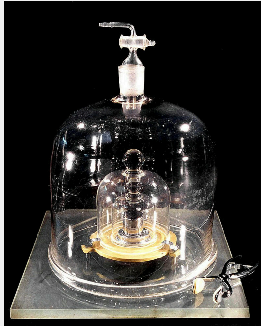
Figure 2.45: The International Prototype of the Kilogram, whose mass was defined to be one kilogram from 1889 to 2019. Picture by BIPM, CC BY-SA 3.0 igo, https://commons.wikimedia.org/w/index.php?curid=117707466
